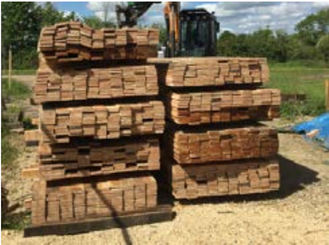
MATERIALS Larch hardwood timber was selected by Antony and Jenni for the shou sugi ban charred timber cladding.
